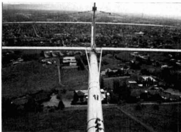
fig. 1. Sighting along boom of a KLM 4 element Yagi reveals unobstructed near field topography.
